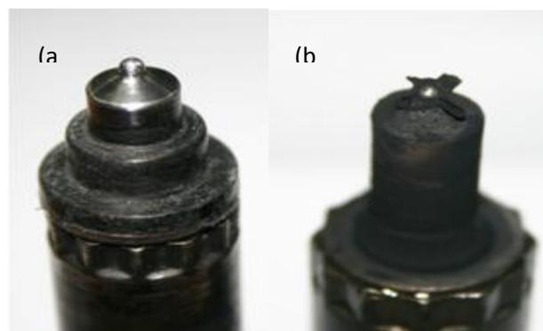
Fig 6. Carbon depositions in Injector tip after using a) No. 2 Diesel b) 95% No. 2 diesel & 5% palm olein.
