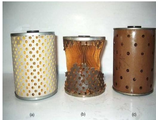
Fig 5 External view of a new fine porous filter element (a) that was damaged during experiments by pure rapeseed oil (b) in comparison with reinforced fielem (c) suitable to withstand oil pressure.
