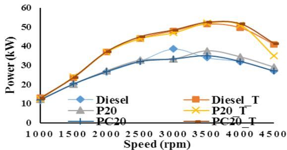
Fig. 3: Engine brake power at different speed
