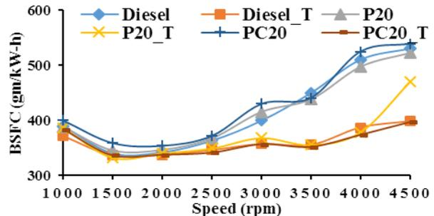
Fig. 4: Engine BSFC at different speed
