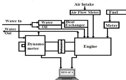
Fig. 1: Schematic of engine test bed
