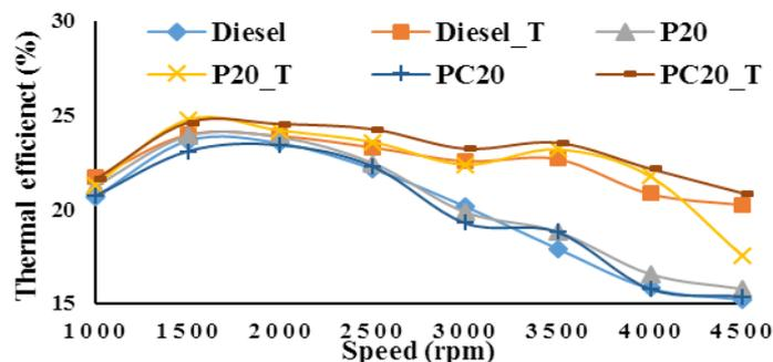
Fig. 5: Engine brake thermal efficiency at different speed
