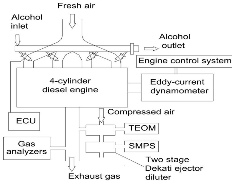
Fig 1: Schematic of experimental setup of alcohol fumigation system
