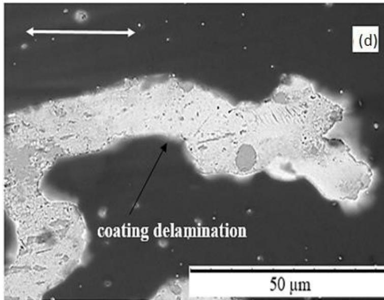
Figure 2. SEM image of un-textured DLC of TMP-C125
