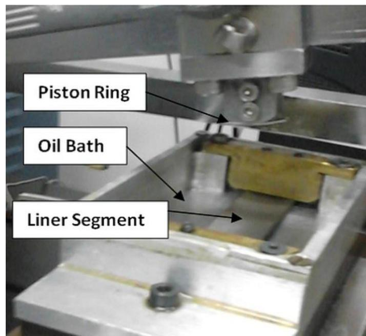
**Fig. 8.** Piston ring and liner specimen in reciprocating test rig
