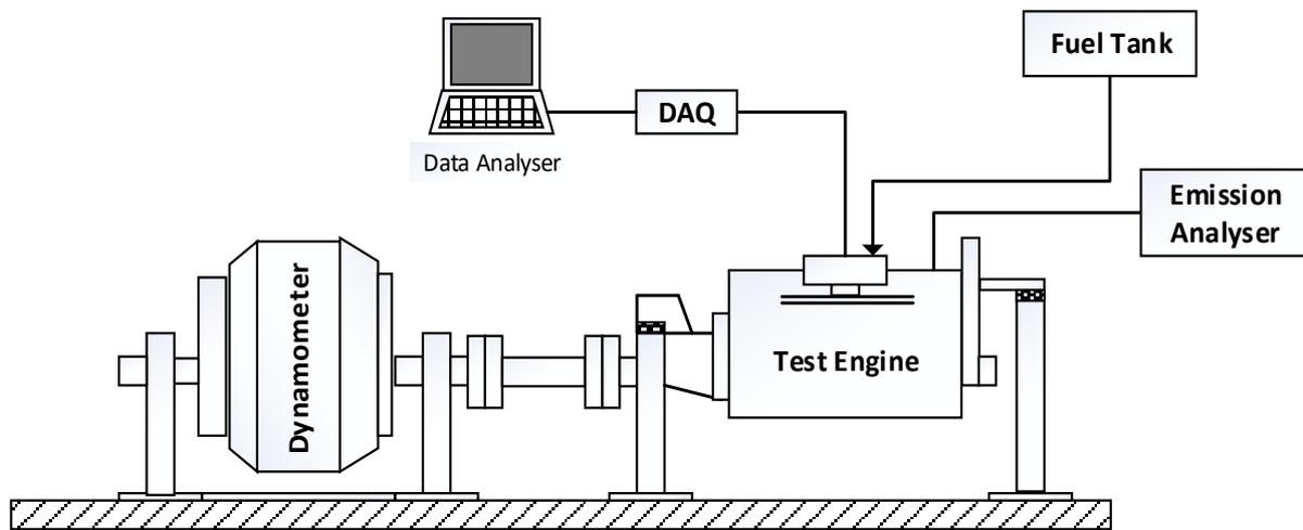
**Fig. 4.** Schematics of the engine test bench
