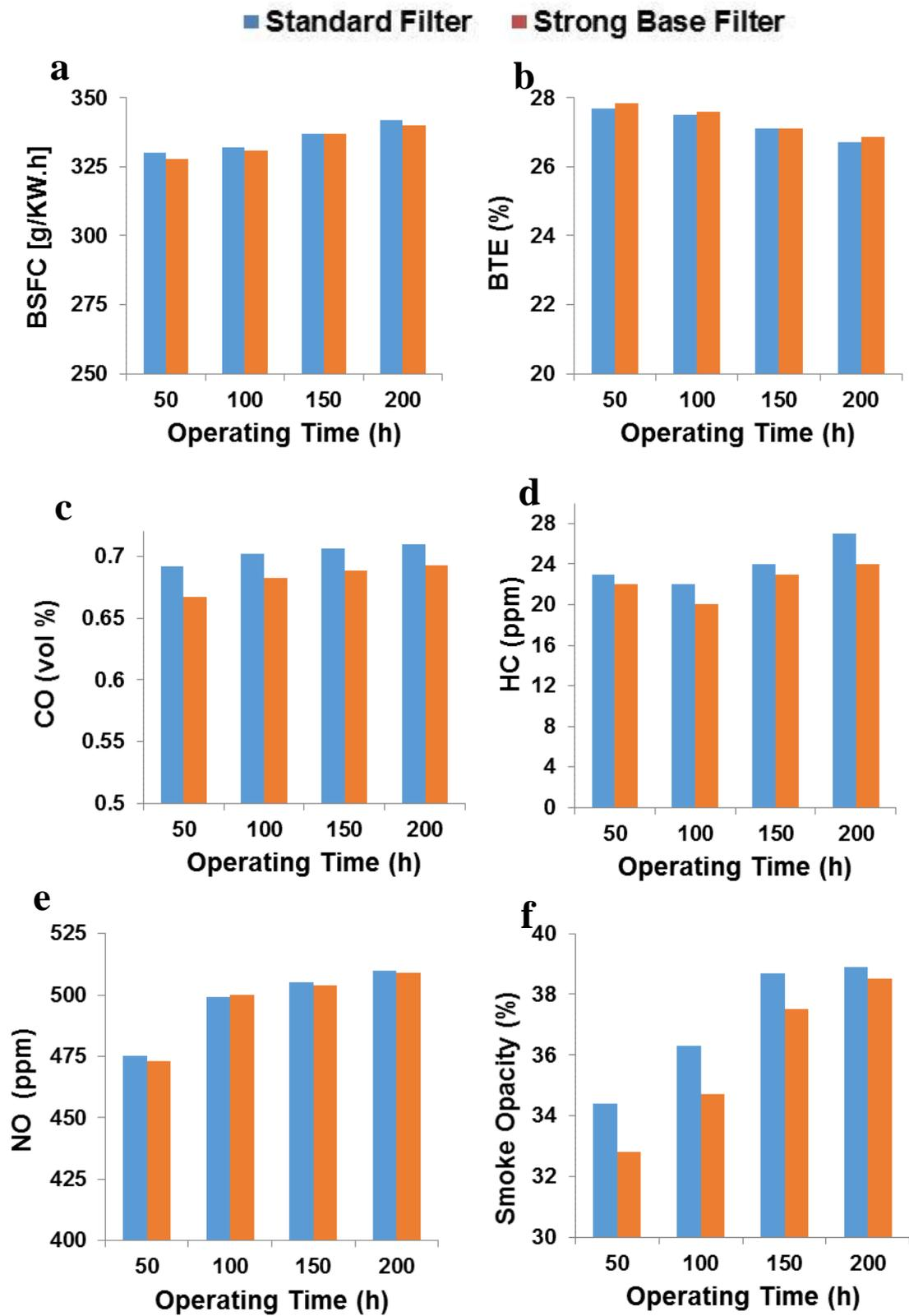
**Fig.10.** Fuel consumption and exhaust emissions during the long hour tests.
