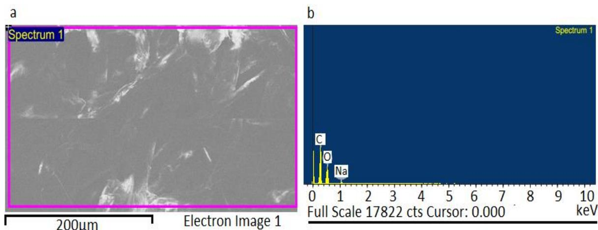
**Fig. 3.** (a) SEM analysis of strong base filter paper (b) EDX analysis showing elemental details
