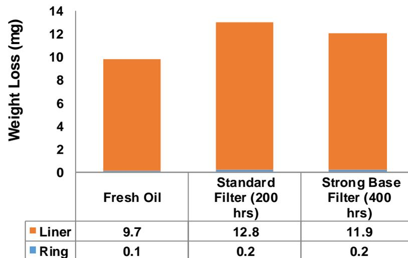
**Fig. 9.** Piston ring and cylinder wear
