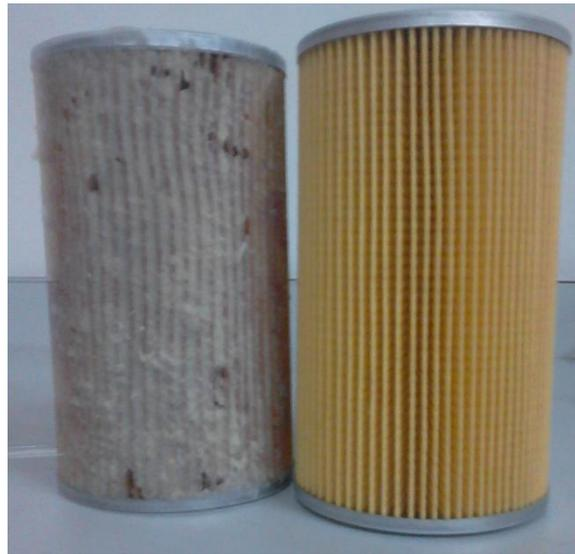
**Fig. 2.** Standard filter element and strong base (NaOH) filter element
