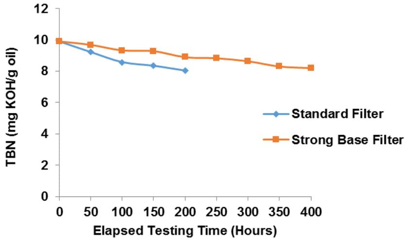
**Fig.5.** TBN retention of degraded oils after long hour tests
